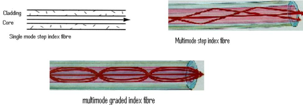
Single-mode fibre is preferred in modern telecommunications because they are digital and use monochromatic laser light. Here the transmission is free from dispersion, and can carry 14 TV channels & 1400 phone calls at the same time.
